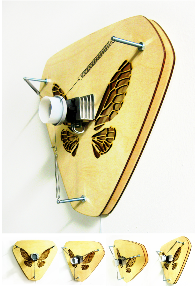
Figure B-1: Custom built 1-bit instrument. The instrument comprises a wooden base, a dot matrix print head, a plastic cap, wire and springs.
